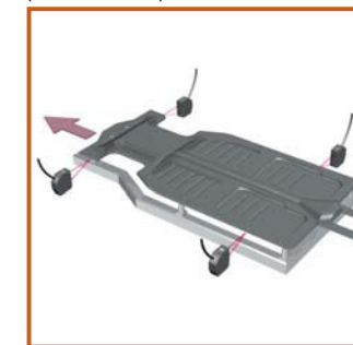
Measuring Car Body Widths (ZS-HLDS10)
